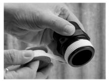
1. Apply PTFE tape or approved sealant to the male thread the blue handled ball valve is to be screwed in too. Sufficient tape needs to be applied to ensure a watertight seal
