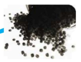
Produce with high performance polypropylene with corrosion, biological and chemical resistant complied to BS6920
